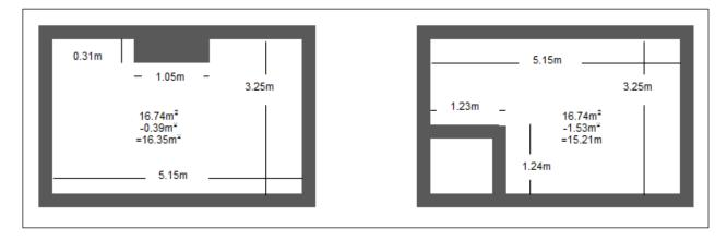
When calculating the floor area of a room that is in, for example, a converted loft, any floor space that has a head-height of less than 1.53m should not be included as illustrated here.
