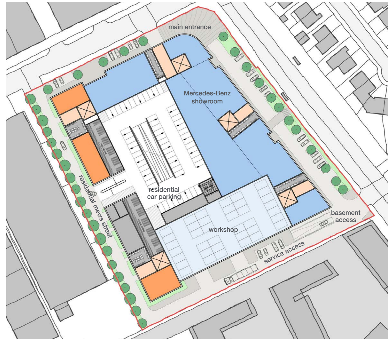
Proposed ground floor plan (commercial frontage, residential mews and podium car parking)
