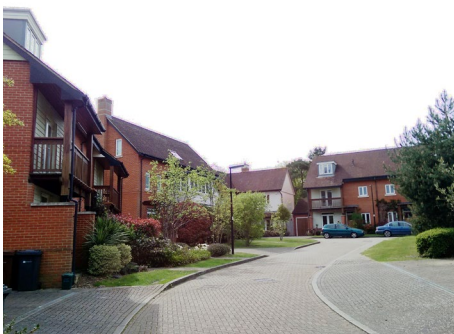
A local street that emphasises pedestrian priority through its surface materials and lack of kerbs ✓
