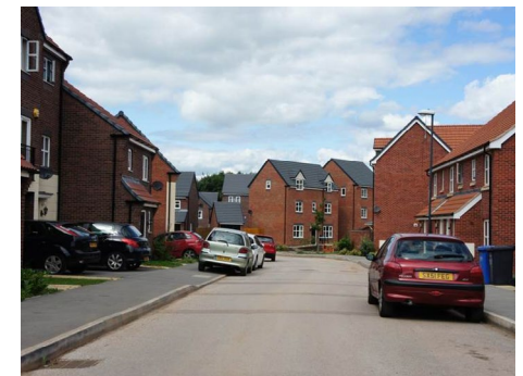
On-street parking is preferred by residents but if not designed in it causes problems ❌
