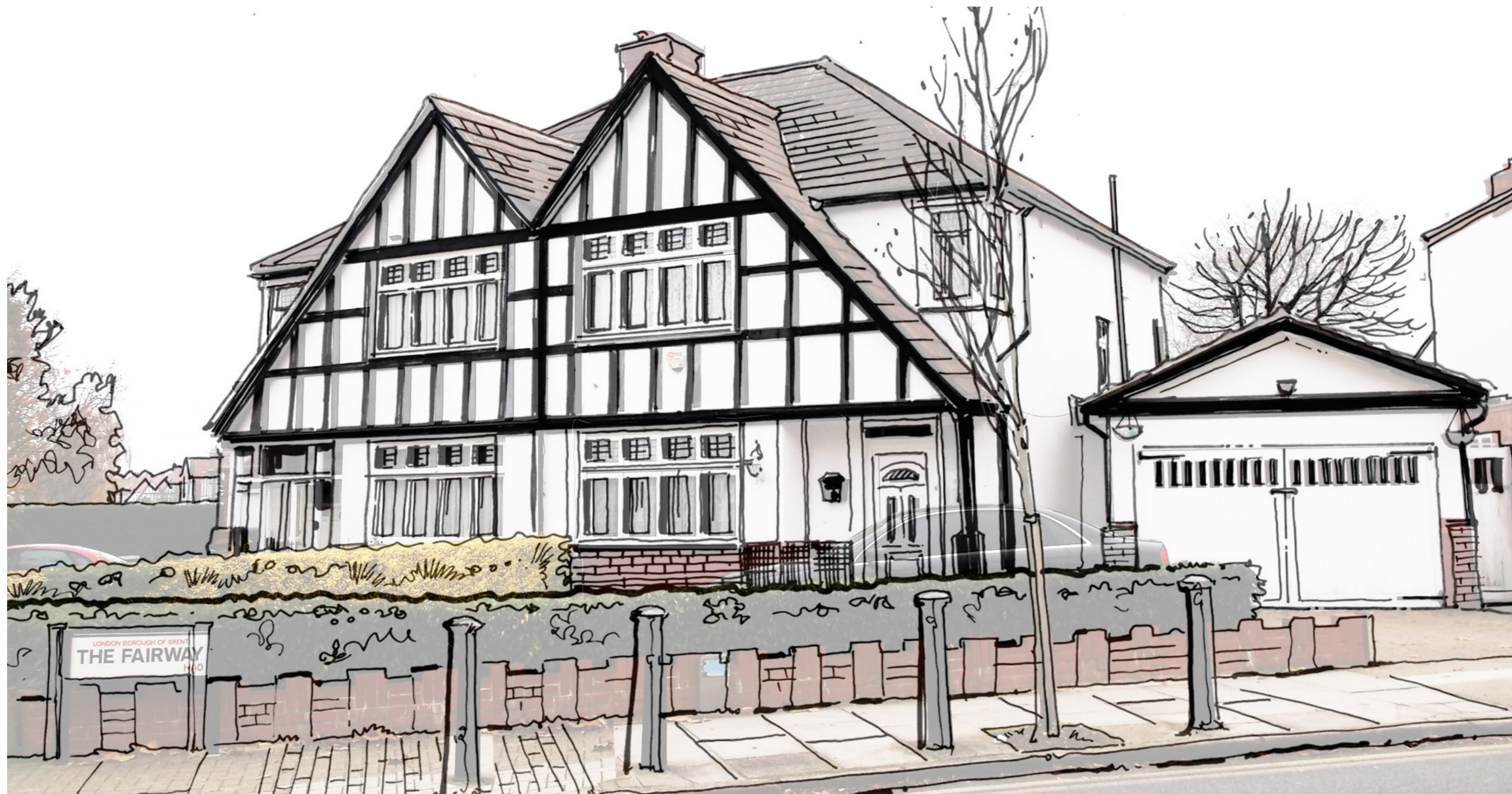
Figure 21: Illustrations of a garage on a side plot. The garage is detached from the house and has side hung timber doors
