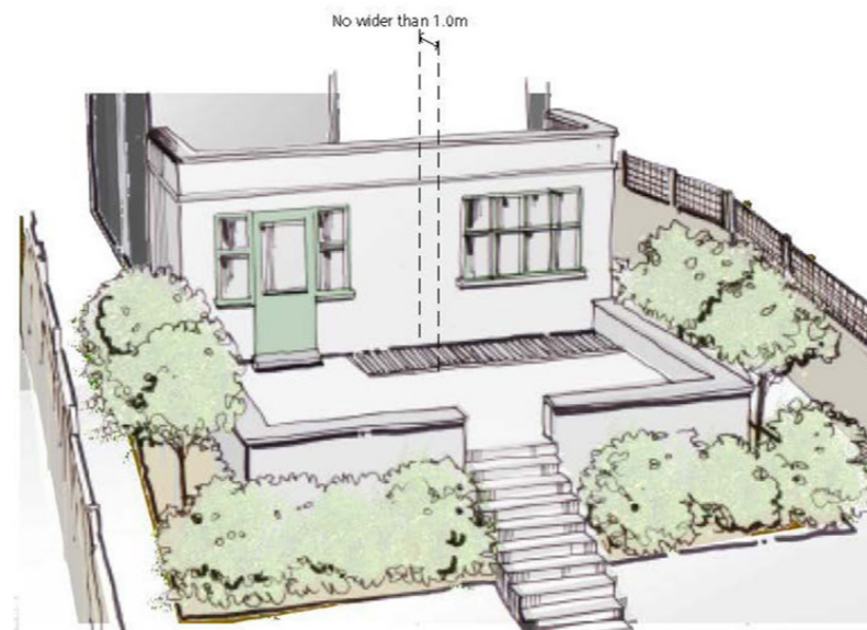
Figure 6: Illustration of a light well concealed in a raised patio or terrace
