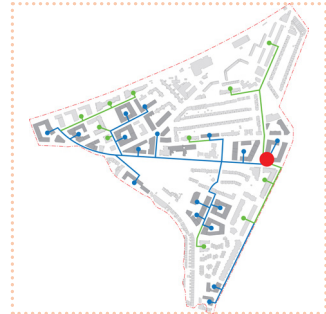
Option B - Proposal for an energy centre covering the entire South Kilburn Regeneration Area
