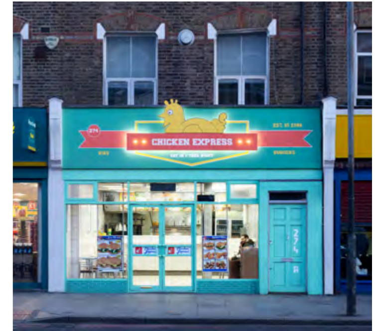
✔ AFTER: New fascia signage restores original building proportions with unique, colourful graphics and considered illumination. The residential entrance reads clearly in subservience to the shop frontage, while de-cluttered glazing allows views into the shop.
